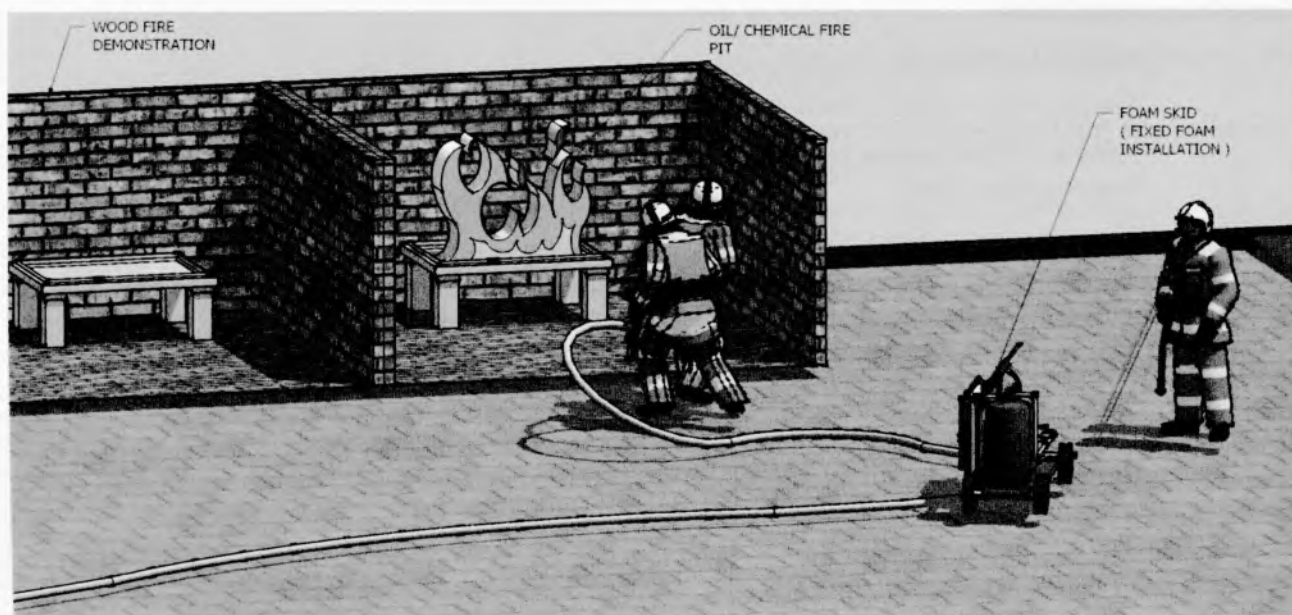
Figure 2 – Oil/chemical fire pit view and demonstration of extinguishing of fire by using fixed foam system
