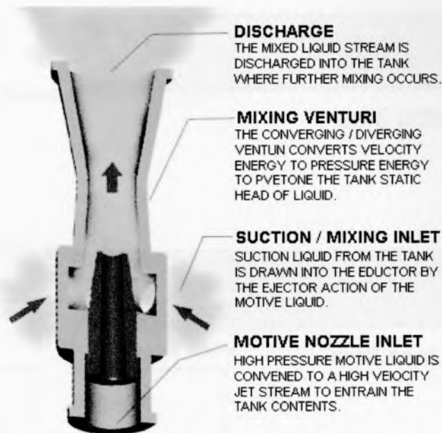
Figure 1.4 A – Eductor used for stripping oil tanks
